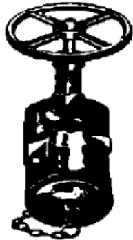
fire pump Delivery valve.
