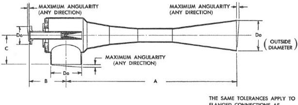
THE SAME TOLERANCES APPLY TO FLANGED CONNECTIONS AS ARE SHOWN FOR BUTT WELDED CONNECTIONS
