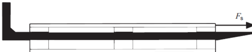
STATIC COEFFICIENT OF FRICTION TEST
