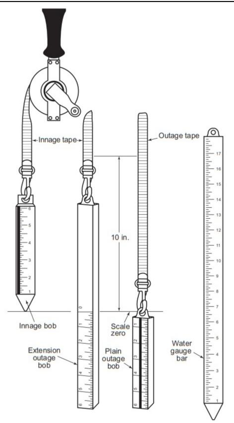
(A) TYPICAL GAUGE TAPES AND BOBS (B) TYPICAL WATER GAUGE BAR TYPICAL GAUGE TAPES AND BOBS AND TYPICAL WATER GAUGE BAR
