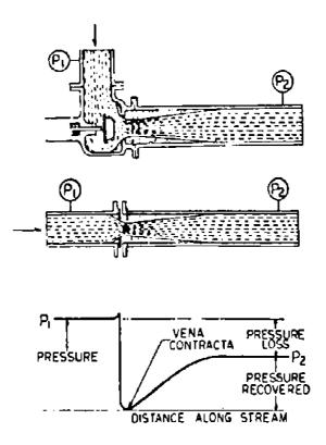
CONTROL VALVE AND ORIFICE PLATE INSTALLATIONS SHOWING REDUCED AREA AT VENA CONTRACTA. THE CURVE DESCRIBES THE PRESSURE GRADIENT AROUND EITHER DEVICE Fig. 1 Neglecting friction and other non-ideal influences for a moment, Bernoulli's theorem tells us that
