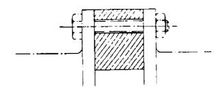
BUTTERFLY VALVE: SINGLE FLANGE WAFER TYPE Fig. 15
