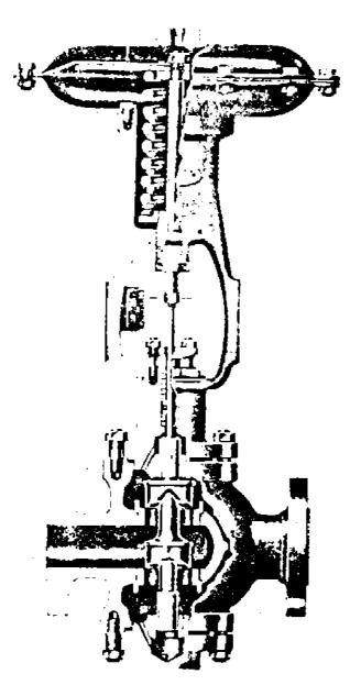
TYPICAL CONTROL VALVE ASSEMBLY Fig. 1
