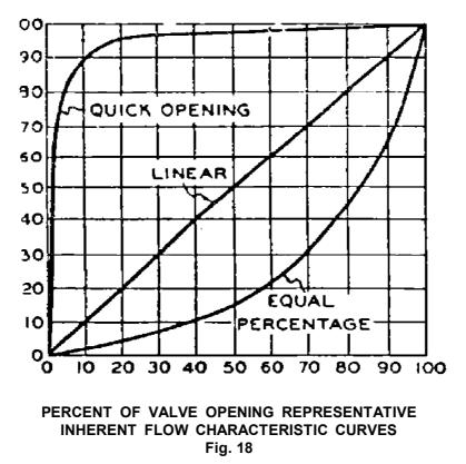
**8.2.1** Characteristic of the inner valve shall normally be equal percentage except where system characteristics indicate otherwise. Linear and quick opening characteristics shall be used where required. In general linear trim shall be used only for Split-Range service or where control valve pressure drop remains constant over the range of 10% to 100% of flow capacity.
