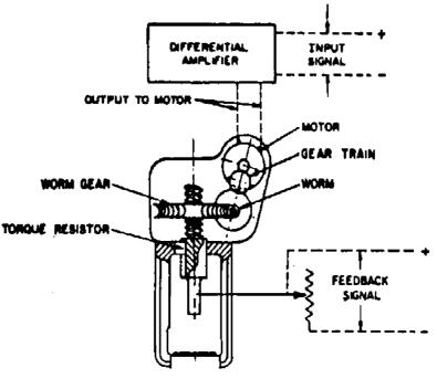
AN ELECTRO-MECHANICAL VALVE ACTUATOR Fig. 21
