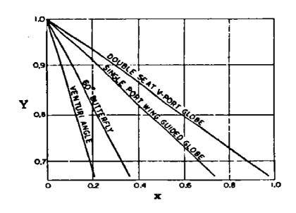
EXPANSION FACTOR, Y AS A FUNCTION OF PRESSURE DROP RATIO, X, FOUR WIDELY DIFFERING STYLES OF CONTROL VALVE Fig. 2
