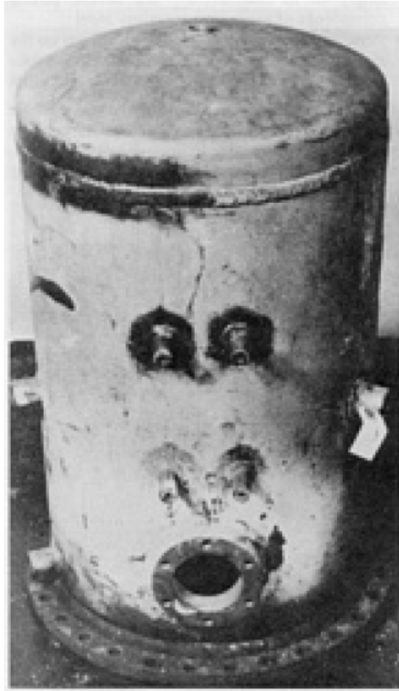
Fig. 7-AS-WELDED TYPE 430 STAINLESS STEEL SATURATOR TANK USED IN THE MANUFACTURE OF CARBONATED WATER THAT FAILED AFTER 2 MONTHS OF SERVICE. THE TANK WAS SHIELDED METAL ARC WELDED USING TYPE E308 STAINLESS STEEL FILLER METAL
