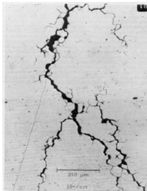
Fig. A.3.3 CAUSTIC SCC IN THE HAZ OF A TYPE 316L STAINLESS STEEL NaOH REACTOR VESSEL. CRACKS ARE BRANCHING AND INTERGRANULAR
