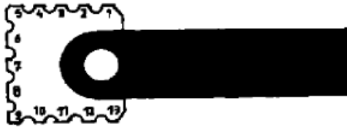
Fig. 3-WET FILM THICKNESS GAGE-MEASURES COATING THICKNESS DURING APPLICATION BY PROGRESSIVELY DEEPER STEPS MARKED IN MILS
